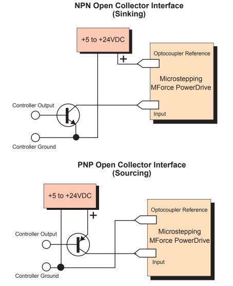
Figure 2.4.5: Open Collector Interface Example
